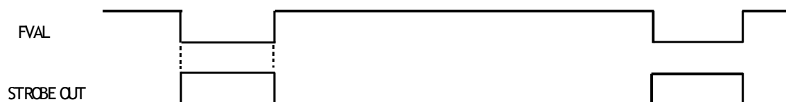
Fig.18. Strobe output timing for Continuous mode
